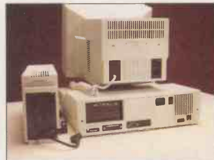
A separate box is required for full-length cards (above) but the power supply is now internal (below).
